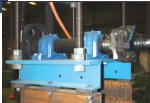
1 - Sealed cross beam connection; 2- Longitudinal rail cleat connection; 3 - Exciter beam flange stress relieved and machined; 4 - Lay shaft drive assembly.
