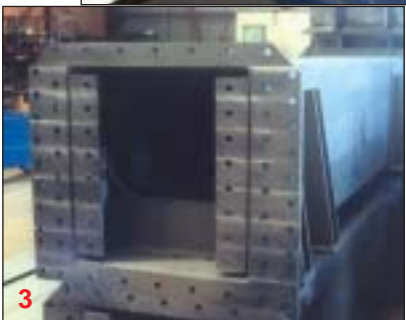
1 - Sealed cross beam connection; 2- Longitudinal rail cleat connection; 3 - Exciter beam flange stress relieved and machined; 4 - Lay shaft drive assembly.
