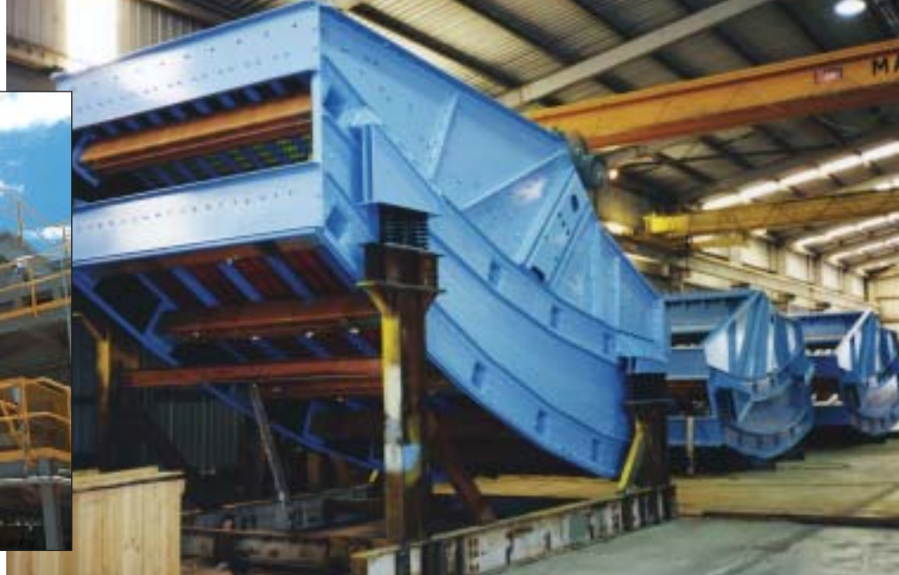
Banana screens being assembled in Schenck works
