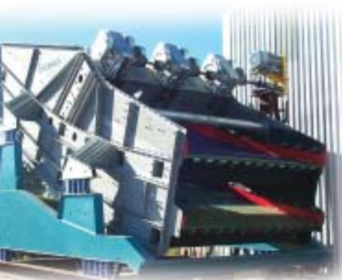
30 ton double deck screen for a diamond mine
