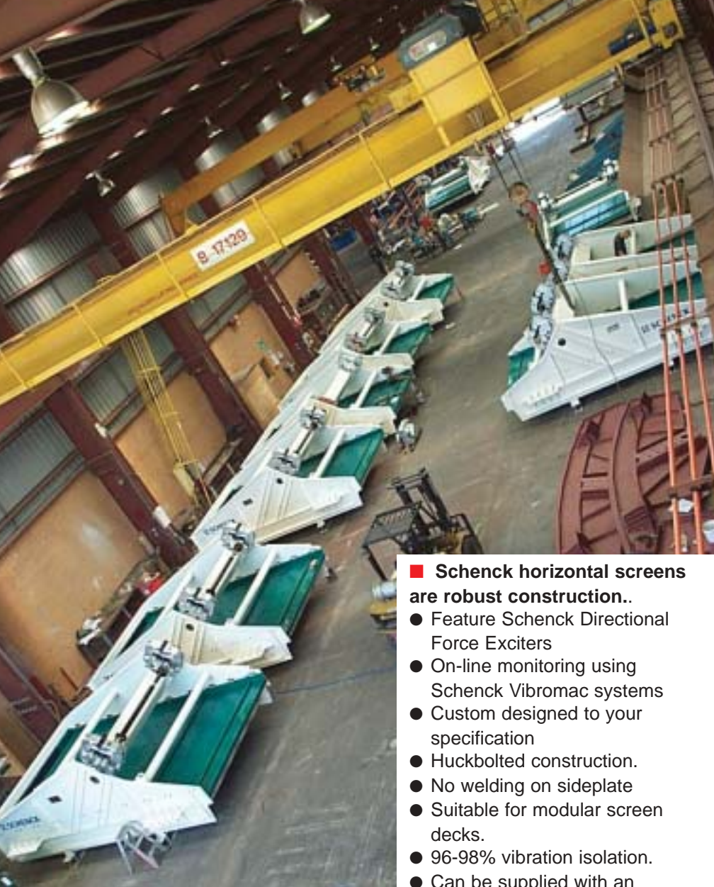
10 Horizontal screens being assembled at Schenck works
