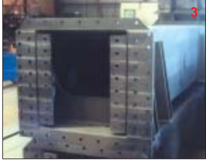
1 - Sealed cross beam connection; 2 - Longitudinal rail cleat connection; 3 - Exciter beam flange stress relieved and machined; 4 - Lay shaft drive assembly.
